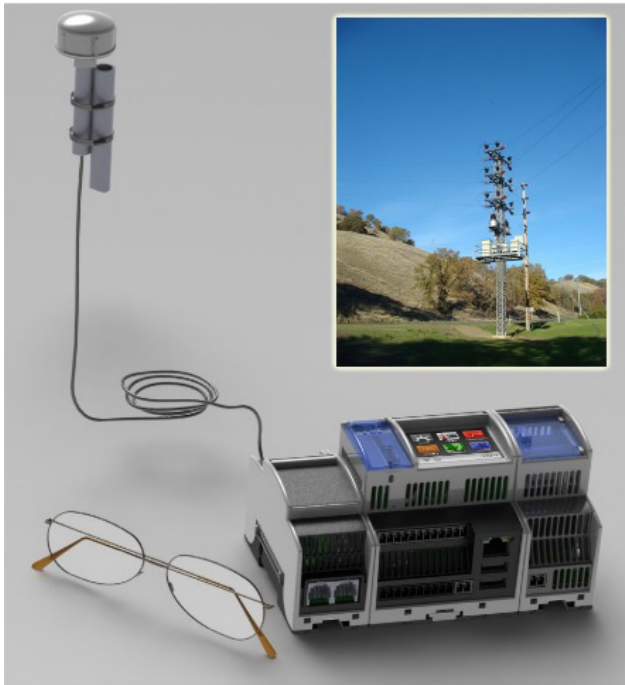
Figure 7. \mu PMU concept (along with size reference) and implementation in the grid around Berkeley.
