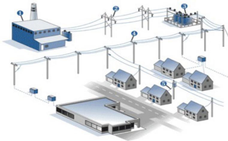
Figure 6. Micro-synchrophasors ( \mu PMU's) at every node in a distribution grid
