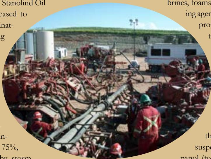
**Modern fracking operations utilize powerful pumps and vast amounts of water and chemicals to liberate trapped gases and oils.**
